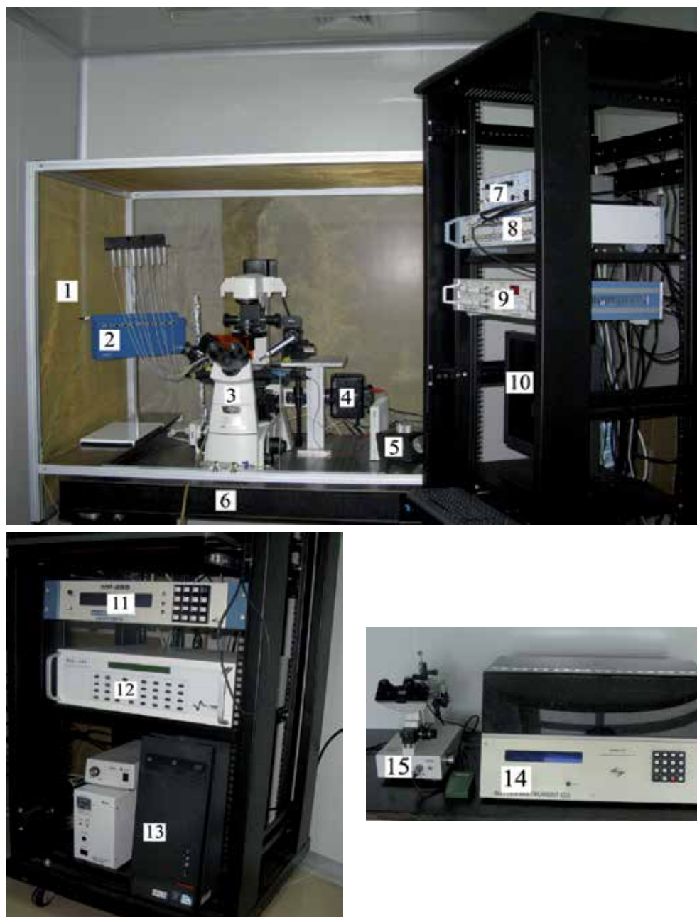
Fig. 2. A conventional patch clamp setup comprising of 1) Faraday cage; 2) Solution perfusion system (EVH-9); 3) Inverted microscope; 4) CCD camera; 5) Motorized micromanipulator controller; 6) Air suspension table; 7) Temperature controller; 8) Digidata; 9) Amplifier (Axopatch 200B); 10) Computer display; 11) Micromanipulator; 12) Rapid solution changer command box (RSC-200); 13) Computer monitor; 14) Micropipette puller; 15) Micropipette Beveler.
