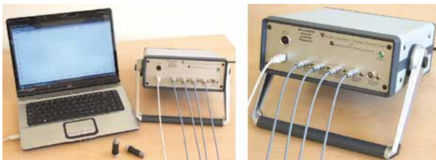
Fig. 16. Commercial-like measurement system driving 5 discreet pressure sensors
