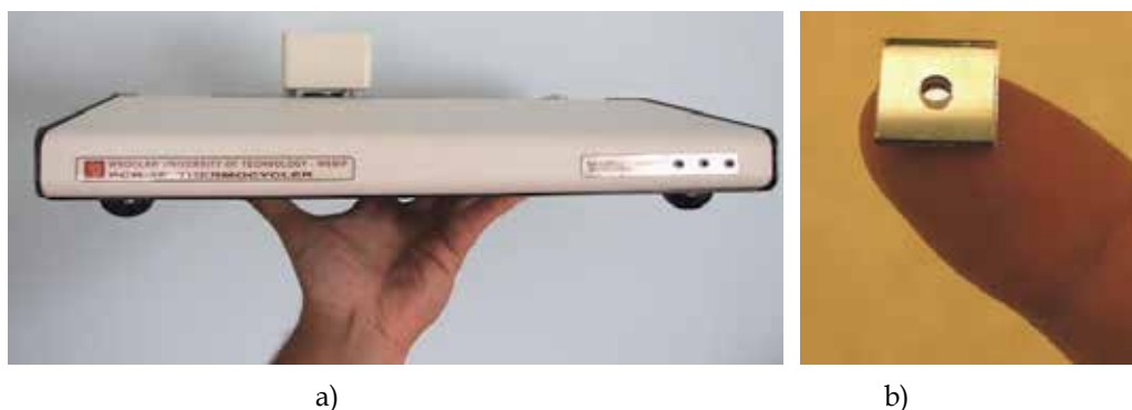
Fig. 37. Desktop real-time PCR device co-working with silicon-glass reusable chips: a) view of the instrument, b) 1 cm x 1 cm chip on author's finger
