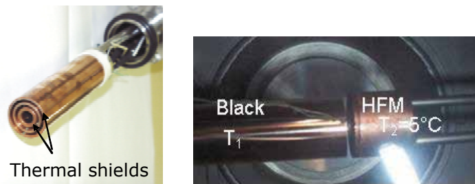
Fig. 2. Picture of the black body (left) and top view of the calibration experiment (right)
