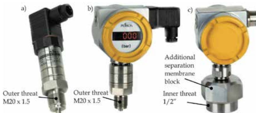
Fig. 3. Examples of commercially available pressure transducers (Peltron, Poland) with stainless steel separation membrane: a) NPX series, b) PXW series with LED display, c) PXC series with additional separation membrane dedicated to harsh environment measurements.
