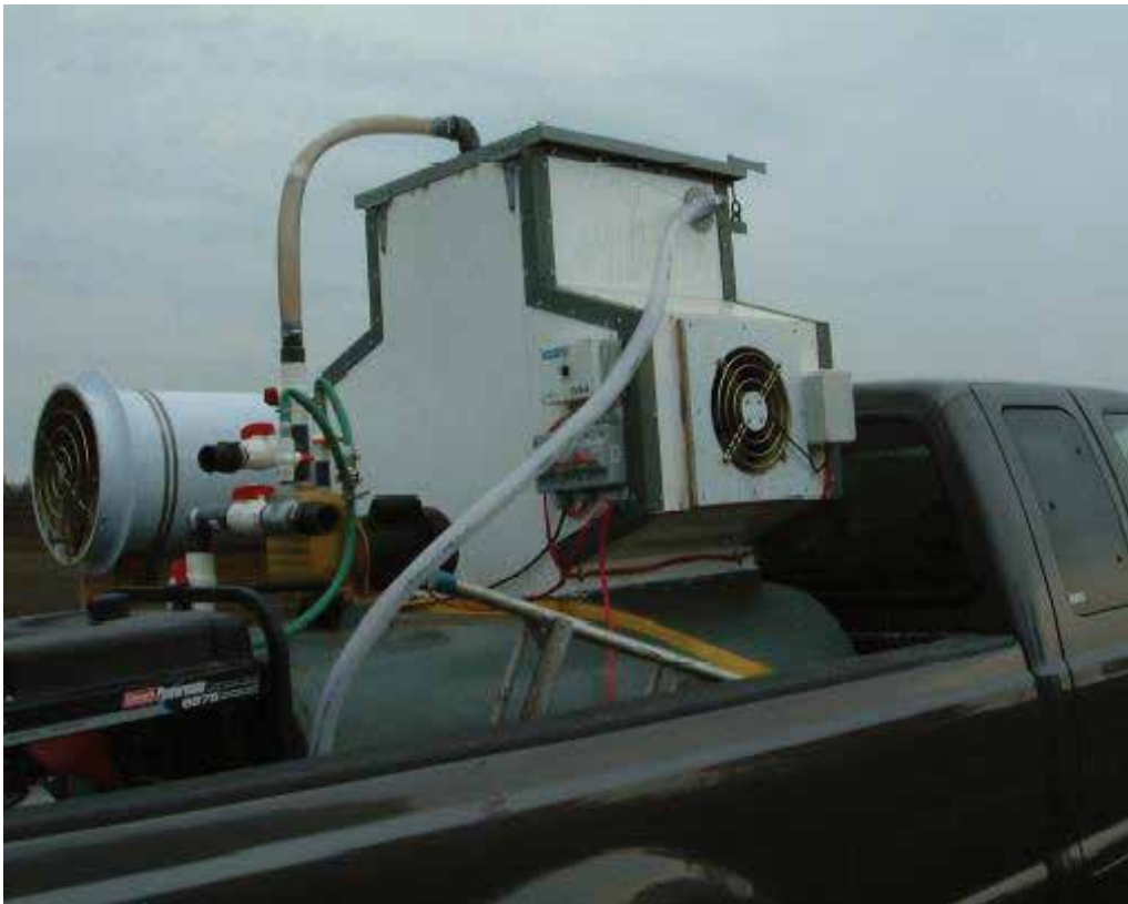
Fig. 1. The odour generator carried on a truck to be positioned at specific distances upwind from the windbreak (Lin et al., 2006)
