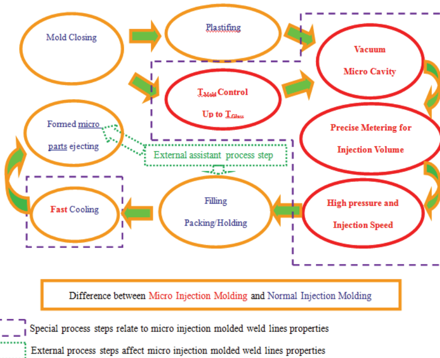
Fig. 1-2. Micro injection molding processing steps
