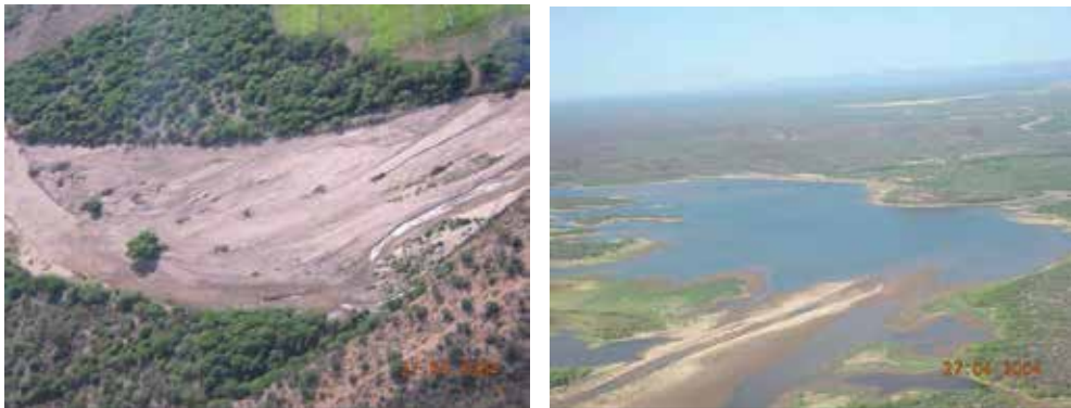
Fig. 10. Evidence of silting up in the Matapé River bed: 10a (left) a general widening and enhancement of river bed is observed; 10b (right) downstream, sedimentation is filling the dams reservoirs, threatening the irrigation downstream in the Coastal, semi-arid, plain.
