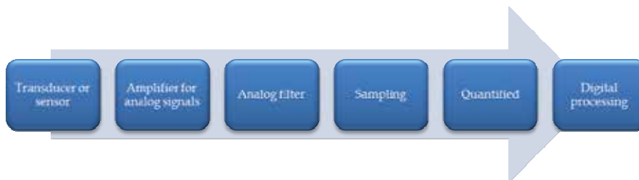
Fig. 6. General block diagram of a procedure analogue to digital (Bronzino, 1999)
