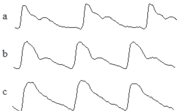
Fig. 8. Wrist cuff waveforms reflecting age differences.
