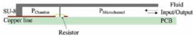
Fig. 16. Cross-section view of the 2D micro impulsion device. Pressure in the chamber is regulated through a PCB orifice.
