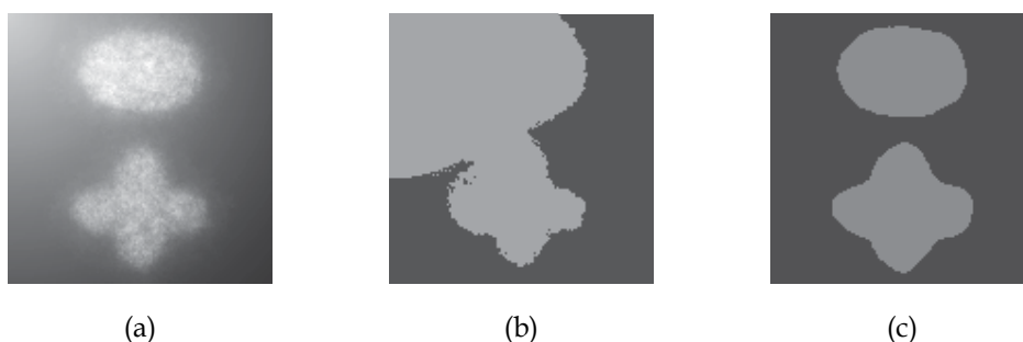
Fig. 12. Segmentation results on the first synthetic image. (a) The synthetic image generated by MOSE. (b) Segmentation by FCM. (c) Segmentation by 2DFCM.
