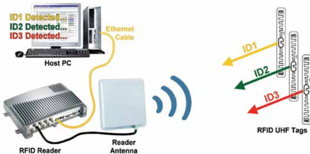
Fig. 1. Schematization of an RFID System
