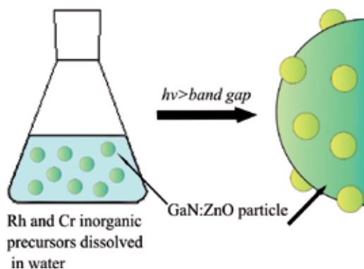
Fig. 7. Scheme showing the photoconversion of inorganic precursors of Rh and Cr and their deposition of particles of GaN:ZnO. After from Maeda et al., 2008
