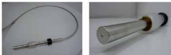
Fig. 1. Mid-IR fibre and ATR probe (left) and IR probe focused on the ATR element (right).
