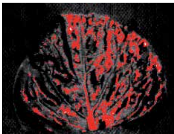
Fig. 9. ROI image of the sample with the chlorpyrifos concentration of 8mg/kg sample.
