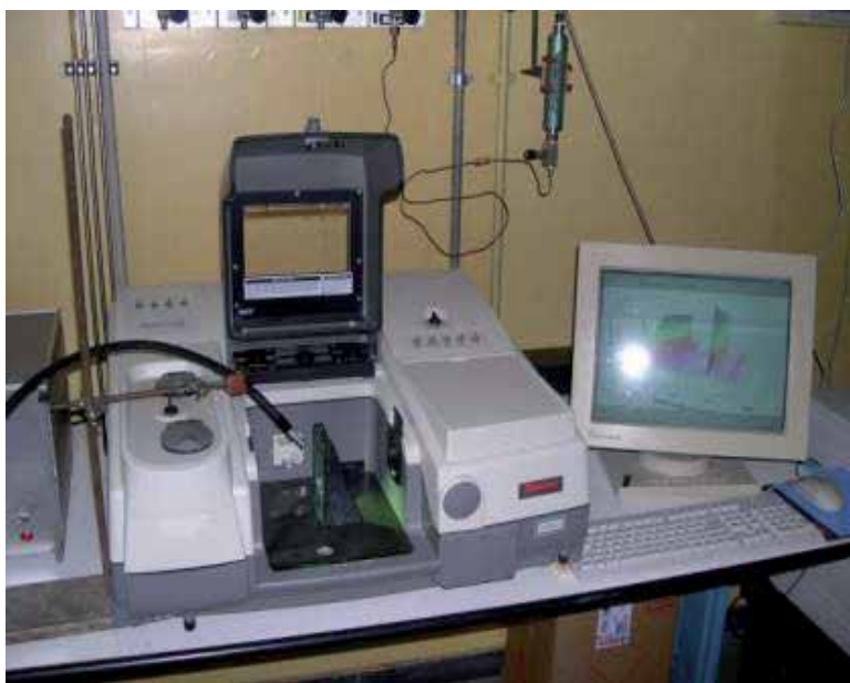
Fig. 1. Set up for RT-FTIR monitoring of UV irradiation curing
