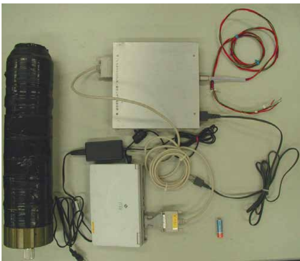
Plate 1. Deep sea gamma-ray sensor for a manned submersible Shinkai6500 . NaI(Tl) scintillator are in the Al-pressure container (dark green colour, wrapped by black plastic tape, left). Under an operation, the sensor unit is connected thorough an underwater connector on the pressure container (silver coloured cover) to a feed-through on the pressure hull of submersible by underwater cable. The data signals are transferred to PC via power supply box (silver coloured) where +12V DC power is converted from AC power supplied from submersible to feed to the sensor unit.
