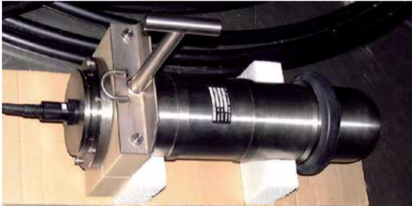
Plate 2. Gamma ray sensor of cabled observatory off Hatsushima Island.
