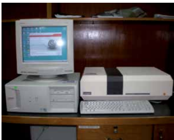
Fig. 3. The UV-visible spectrophotometer model Camspec M530. Faculty of Science, Department of Physics-UPM
