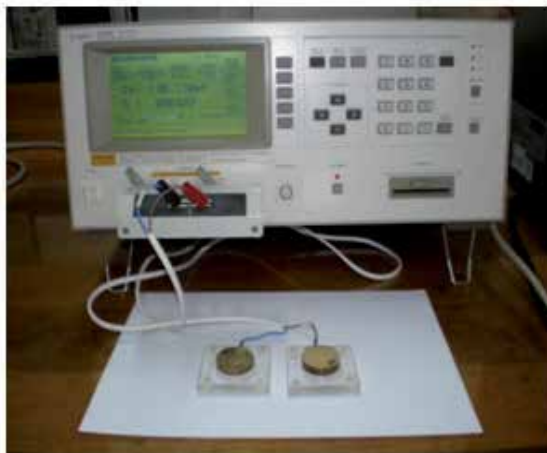
Fig. 5. The LCR-meter model HP 4284A with the sample set up for conductivity measurement. Faculty of Science, department of Physics - UPM
