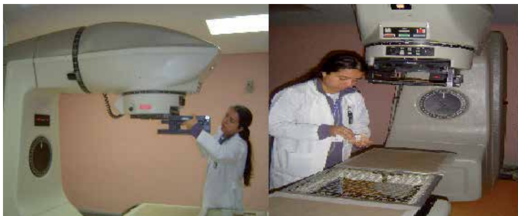
Fig. 1. Cobalt 60 Unit (Theraton 780e), used for irradiation of seeds of Abies religiosa and Pinus hartwegii , located in Centro Estatal de Cancerología de Xalapa, Veracruz, Mex.
