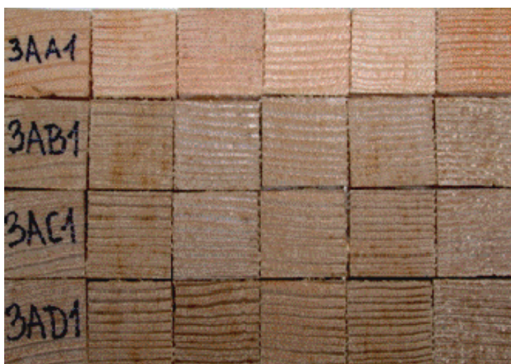
Fig. 4. Colour change of specimens used for mass loss determination, 3AA – control group, 3AB – group irradiated with 30 kGy, 3AC – group irradiated with 90 kGy and 3AD – group of specimens irradiated with 150 kGy.
