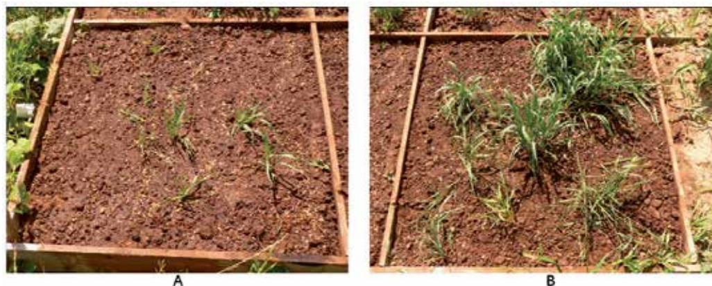
Fig. 11. Pilot testing: soil phytotoxicity evaluation. June, 2007. A – Control plot (soil with oil), B – Plot 4 pre-treated with the consortium "MicroBak" and a fertilizer
