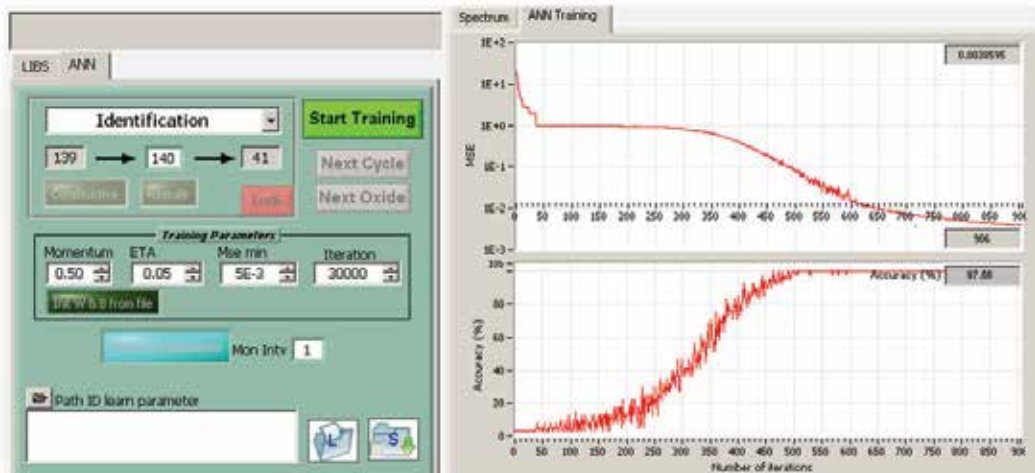
Fig. 9. Identification algorithm programmed in the LabView environment: the training phase.
