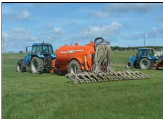
Photo 3. Slurry tanker with trailing shoe application system (Source: Teagasc)
