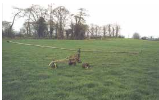
Photo 2. Rotational centre pivot sprinkler system used for dairy dirty water irrigation (Source: www.teagasc.ie )
