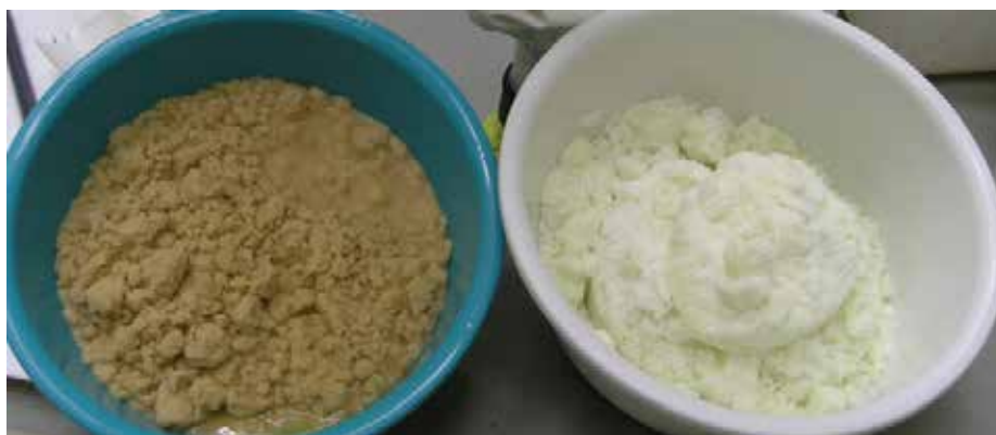
Fig. 4. The separated wet crystals by the original (left) and by the modified (right) technology
