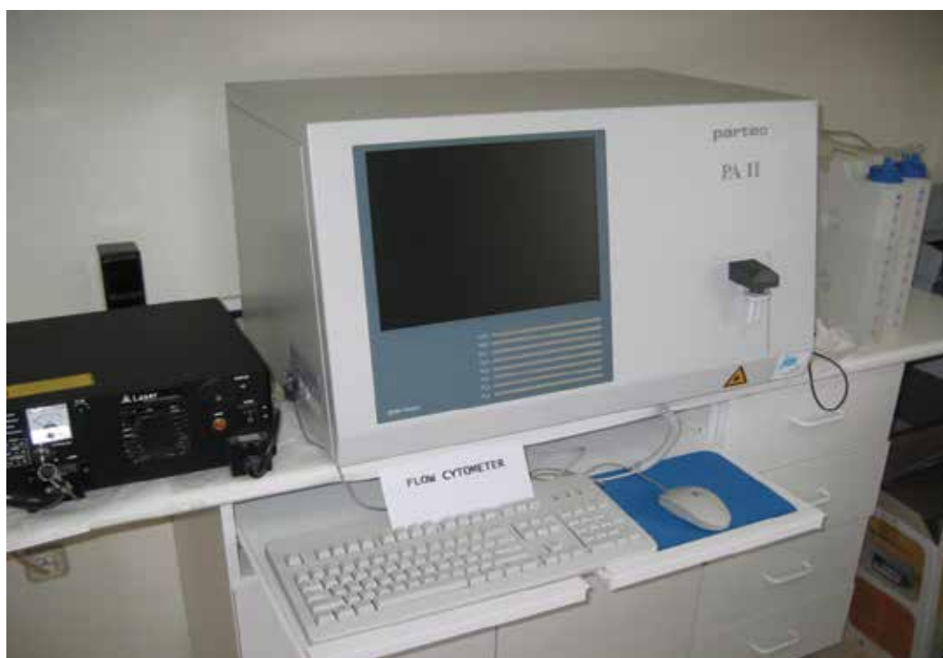
Fig. 2. Flow cytometer used for estimation of nuclear DNA content
