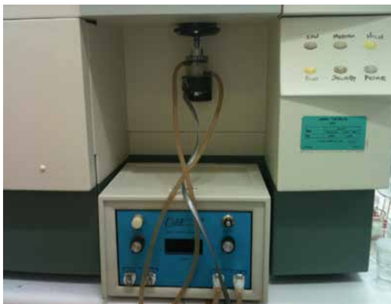
Fig. 1. A picture of Time Zero module integrated with a FACSCalibur flow cytometer
