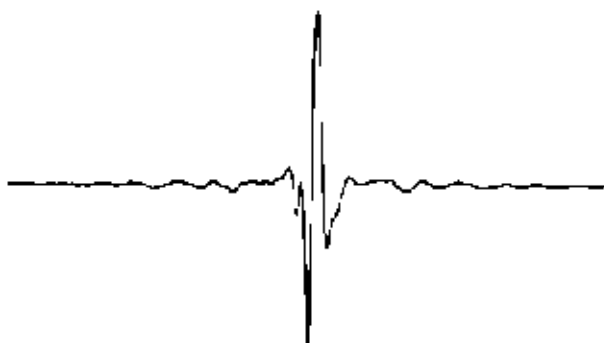
Fig. 2. Typical interferogram (courtesy of Analytical Spectroscopy by R. P. W. Scott, Essential Information for the Analytical chemist http://www.analyticalspectroscopy.net/ )
