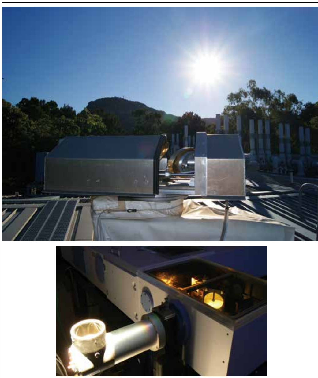
Fig. 1. The ground-based solar Fourier Transform infrared spectrometer at Wollongong, Australia. The sun's radiation is captured by the solar tracker (shown above) and sent to the entrance optics of the high resolution Fourier transform spectrometer in the laboratory below (shown right). (Photography by R Macatangay)
