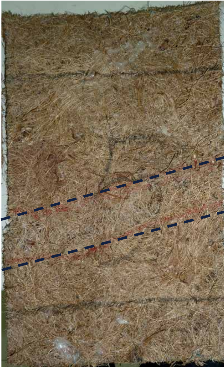
Fig. 13. Rupture area for 5% ABS coated OPEFB sheet
