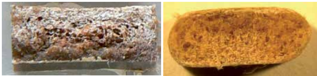
Fig. 30. Cross section of foamed PP filled with 30 wt.% of wood flour - injection molded (left) and extruded profile (right)
