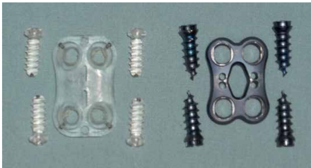
Fig. 4. Resorbable Plate and Screw System (Left) beside Nonresorbable titanium system (Right)
