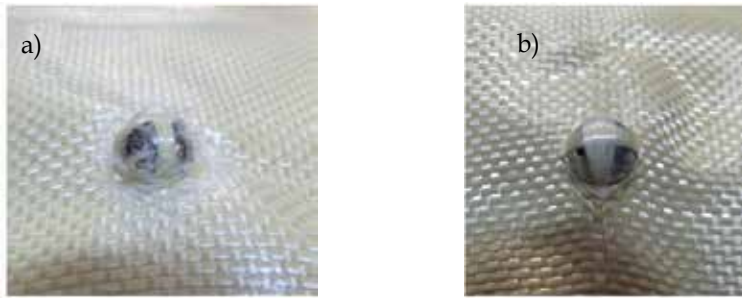
Fig. 4. Aramid samples impacted at different velocities, a) with polypropylene matrix and b) without polypropylene matrix
