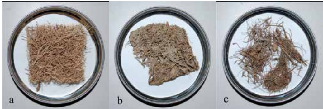
Fig. 17. a) before decay b) decayed ABS coated c) decayed uncoated fibre sheet in the organic clay soil after 3 months
