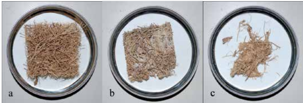
Fig. 16. a) before decay b) decayed ABS coated c) decayed uncoated fibre sheet in the silty sand soil after 3 months
