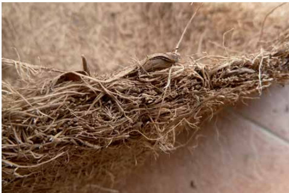
Fig. 10. Longitudinal cross section of OPEFB sheet
