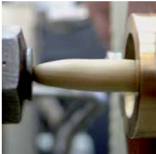
Fig. 33. Extrusion foaming of PP filled with 30 wt.% of wood flour
