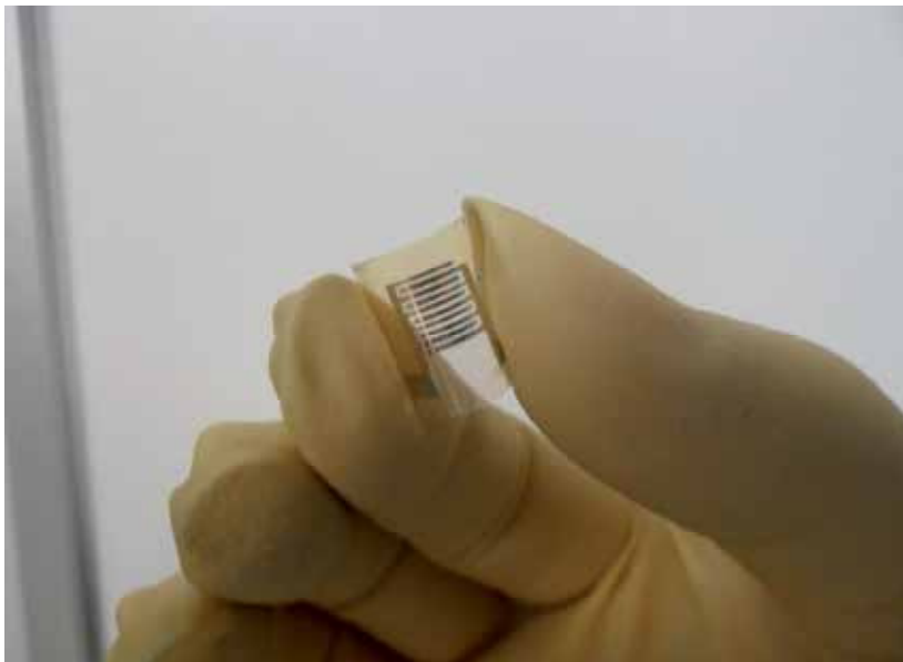
Fig. 12. The ZnO UV PD fabricated on PPC plastic with Pd contacts
