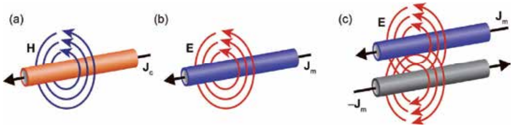
Fig. 4. (a) A schematic illustration of the magnetic-field \mathbf{H} generation from a charge current \mathbf{j}_c according to Ampere's law. (b) A schematic illustration of the electric-field \mathbf{E} generation from a hypothetical magnetic-monopole current \mathbf{j}_m according to the electromagnetic duality and Ampere's law. (c) A schematic illustration of the electric-field \mathbf{E} generation from a pair of hypothetical magnetic-monopole currents, \mathbf{j}_m and -\mathbf{j}_m , or a spin current.
