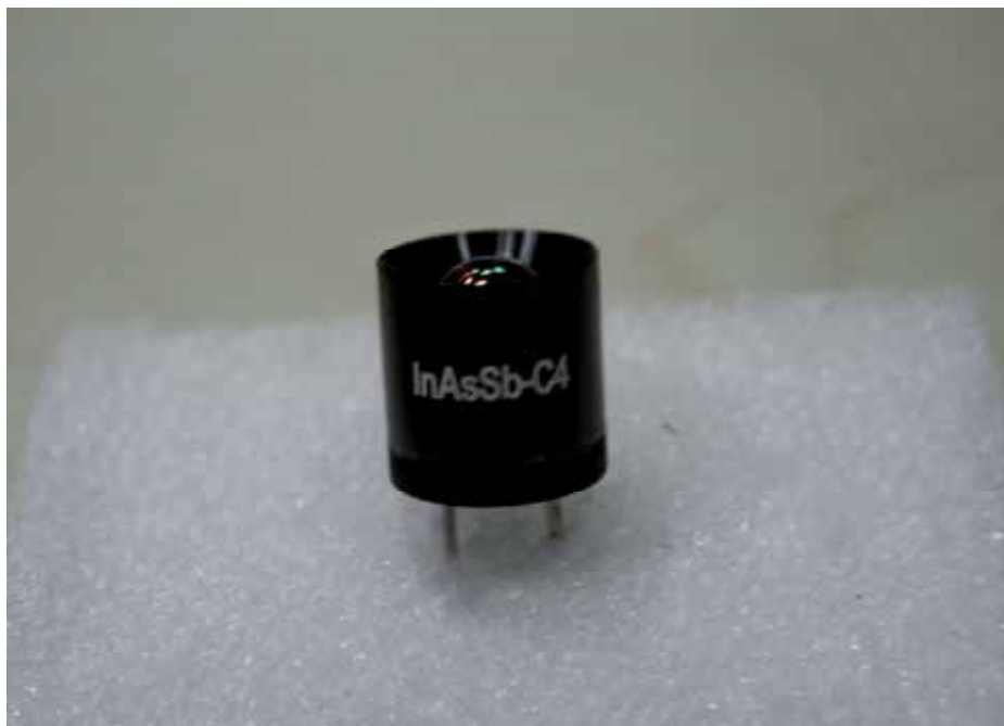
Fig. 9. Photograph of uncooled InAsSb photoconductors.
