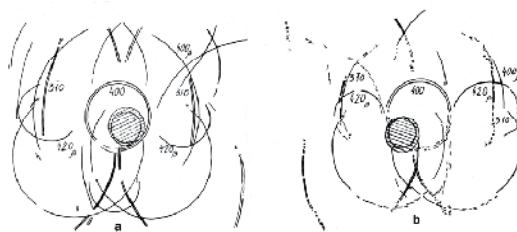
Fig. 9. Divergent X-ray beam patterns of the molybdenum single crystals, grown at rates: a- 0.5 mm/min, b- 6 mm/min.
