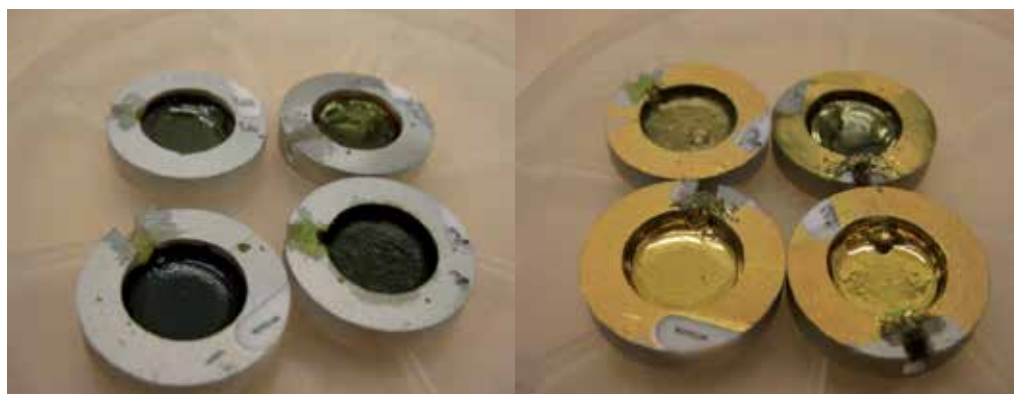
Fig. 9. PbSe NC/MEH-PPH composite assembly deposited on plastic substrates, before the top metal contact is formed (left) and after gold evaporation (right).
