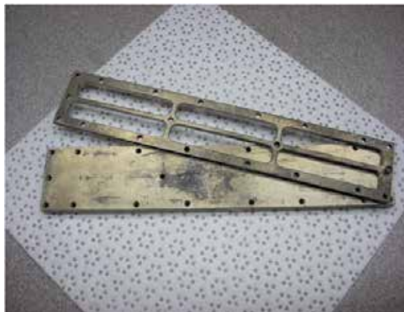
Fig. 1. Stainless steel holder designed to accommodate Kapton samples
