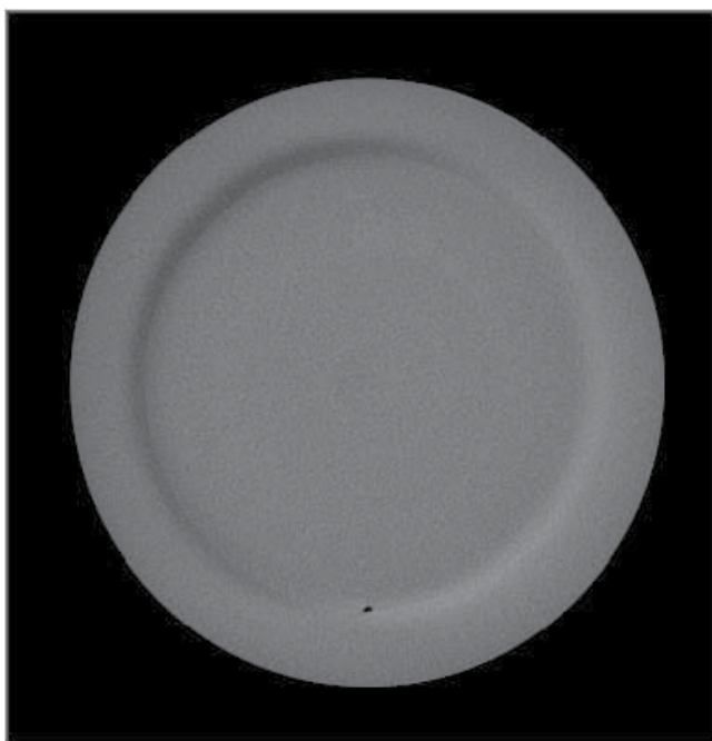
Fig. 13. CBCT image of a slice of the Catphan phantom used to determine Low Contrast Visibility.
