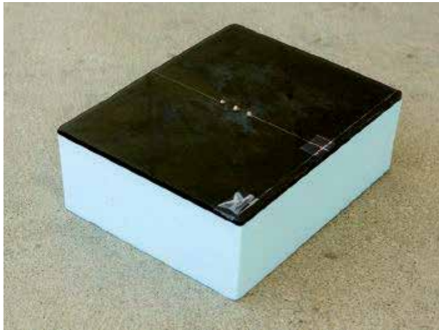
Fig. 2. Simple Level 1 geometry accuracy test phantom. Consisting of three small steel balls (BBs) mounted half-sunken in a Lucite plate on a Styrofoam base, this phantom is used to verify agreement of the isocenters of the kilovoltage and megavoltage beams.
