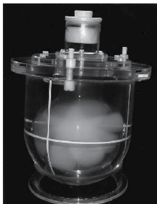
Fig. 5. Phantom used to verify a stereotactically guided conformal treatment plan. (The phantom consists of an inner glass bulb containing the Acrylamide gel, which is surrounded by water in a Perspex container.)
