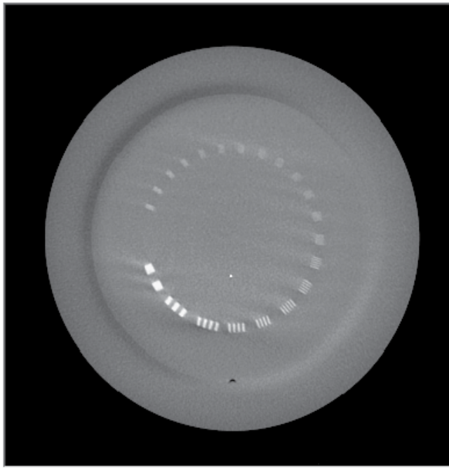
Fig. 11. CBCT image of a slice of the Catphan phantom used to determine the spatial resolution of the imaging system.
