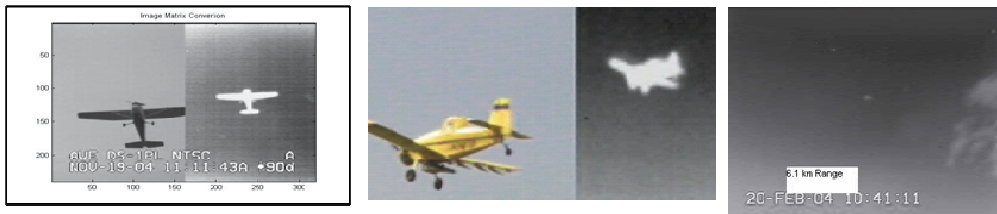
Fig. 8. The detection of single engine Cessna (left), a crop duster (middle) and a twin engine Cessna at 6.1 km (right)
