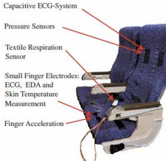
Fig. 1. Airplane seat with integrated unobtrusive sensors [Schumm et al., 2010]
