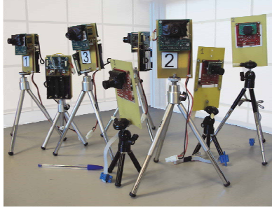
Fig. 5. Set of camera nodes equipped with CMUcam2 and CMUcam3 micro cameras.
