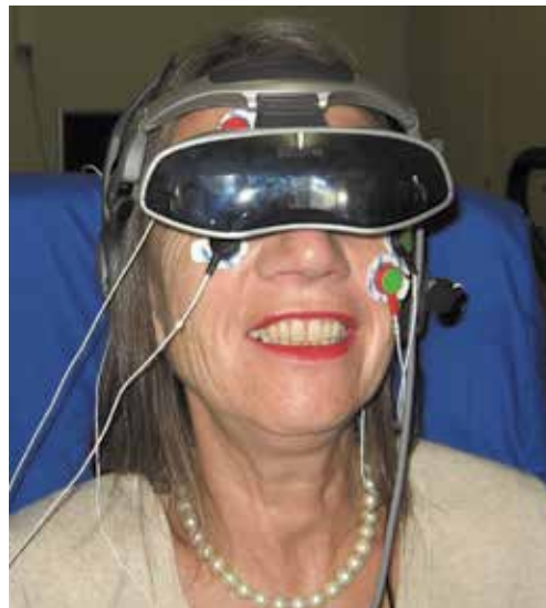
Fig. 8. Subject wearing video glasses to watch emotion eliciting film clips. Vertical EOG and EMG measurement [Schumm et al., 2010].
