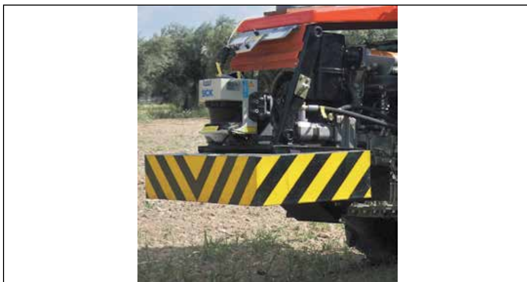
Fig. 2. Detail of the laser range finder and the visual camera.
