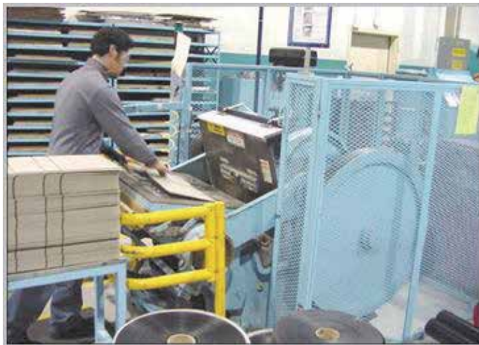
Fig. 24. Press Machine that cuts the BC Bags
