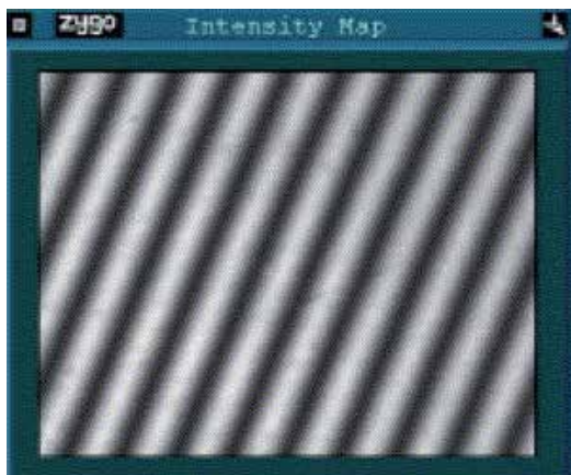
Fig. 2.2. Interference fringe of CBO crystal.
