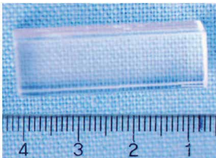
Fig. 4.1. Image of the unprocessed cleavage microchip along the (101) planes directly obtained from the as-grown crystal
