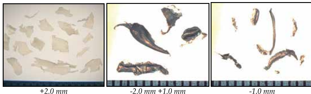
Fig. 14. Bottles in HDPE, images of the products of dry comminution tests.
