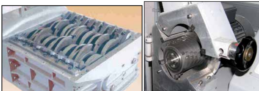
Fig. 6. Industrial shredder blades (left) and comminution chamber of the blade mill adopted in the preliminary tests (right).
