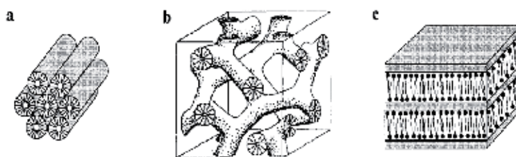
Fig. 3. MCM-41 of hexagonal microstructure (a), MCM-48 of cubic microstructure (b), MCM-50 of lamellar microstructure (c).
