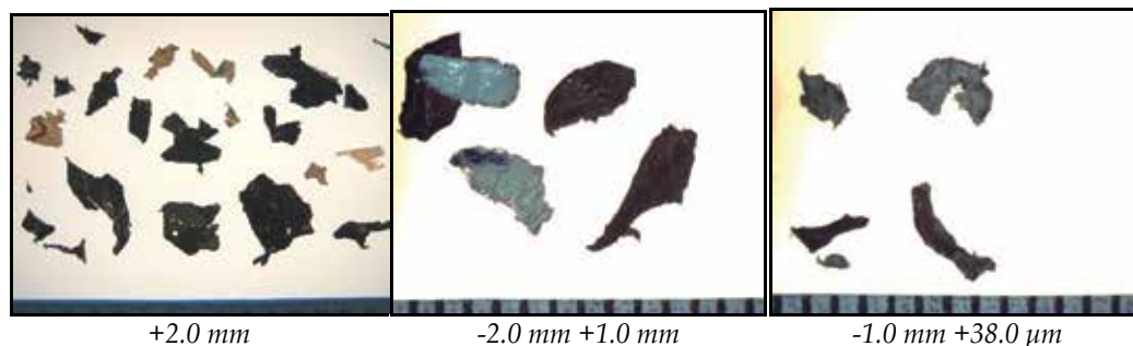
Fig. 18. Bottles in PET, images of the products of dry comminution tests.
