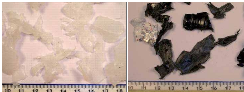
Fig. 7. Comminuted bottles in HDPE (left) and PET (right) obtained in the preliminary tests with the adoption of a 20 mm mesh control grid.
