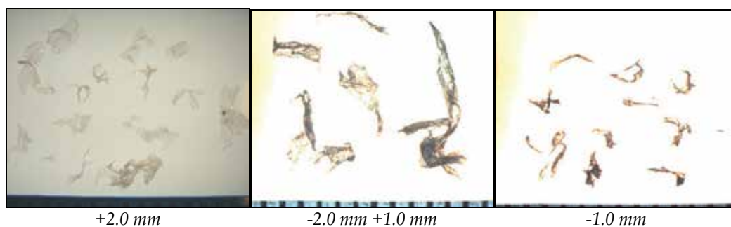
Fig. 23. Plastic bags and films, images of the products of wet comminution tests.
