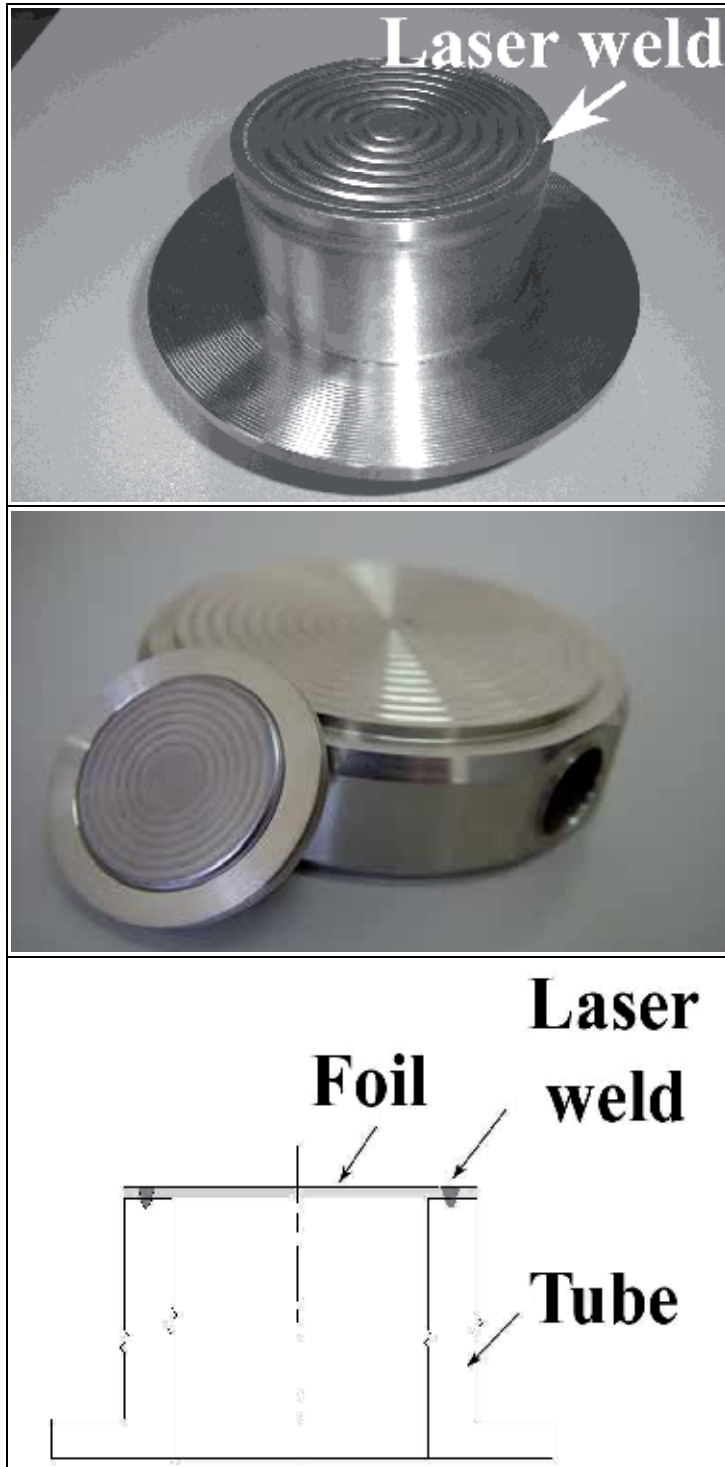
Fig. 1. Chemical seal welded by pulsed Nd:YAG laser.
