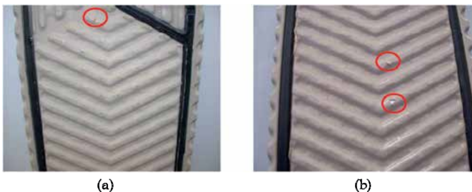
Fig. 14. Coated heat exchanger plates from heating section: (a) A2 coating, (b) A10 coating.
