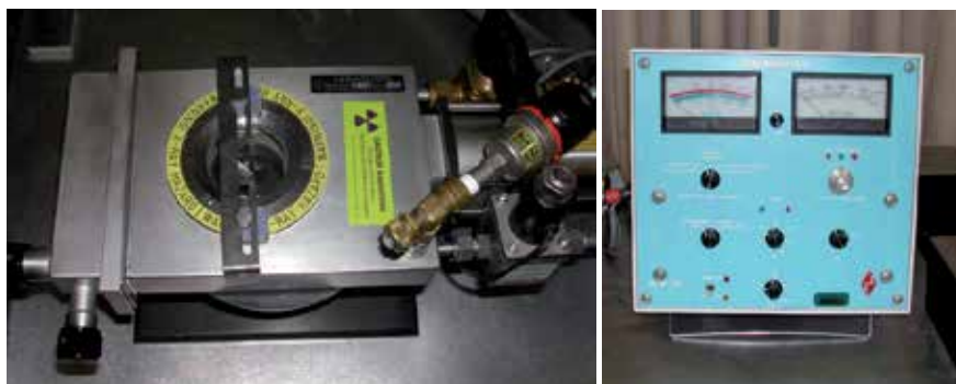
Fig. 2.4. Left: Luminoscope sample holder. Right: Luminoscope control and electronics.
