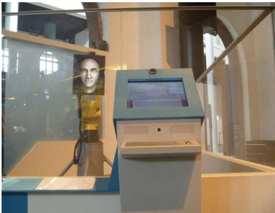
Fig. 7. The information kiosk with the keyboard for language-based interactions with the Articulated Head.
