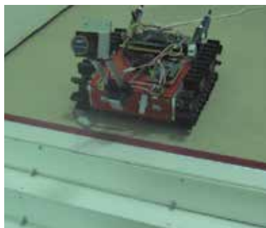
Fig. 8. Overview of an experiment for measurement of downward stairs
