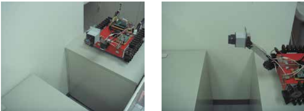
Fig. 11. Overview of an experiment for measurement of a valley configuration (left: front view, right: side view)
