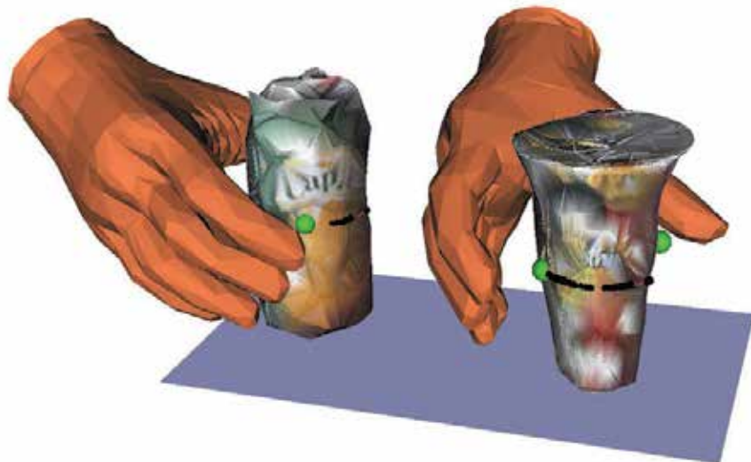
Fig. 9. The rotation axis of the hand is defined by the fingertip of the thumb and the index finger of the gripper. This rotation axis must be aligned with the axis defined by the grasping points. The calculated grasping pose of the gripper is by object no. 8 (Cappy) -32.5^\circ and object no. 9 (Smoothie) -55^\circ .
