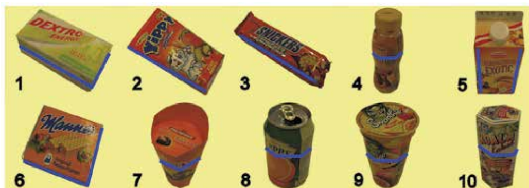
Fig. 11. Ten test objects. The blue lines represent the optimal positions for grasping points near the centre of the objects, depending on the used gripper. From left top: 1. Dextro, 2. Yippi, 3. Snickers, 4. Cafemio, 5. Exotic, 6. Manner, 7. Maroni, 8. Cappy, 9. Smoothie, 10. Koala.
