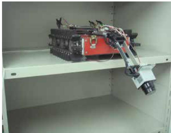
Fig. 14. Overview of an experiment for measurement of a side hole configuration under the robot
