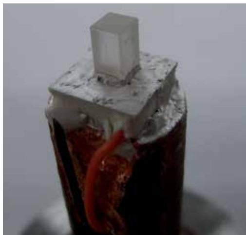
Fig. 10. Pyroelectric crystal, Peltier device, and copper rod, glued by silver paste.
