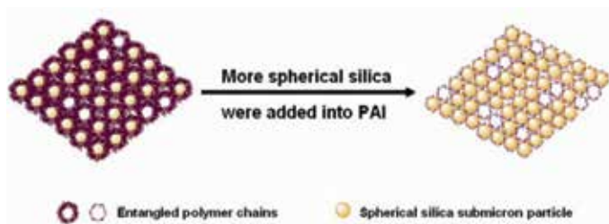
Scheme 3. Interactions between the silica submicron particles and the PAI polymer matrix.
