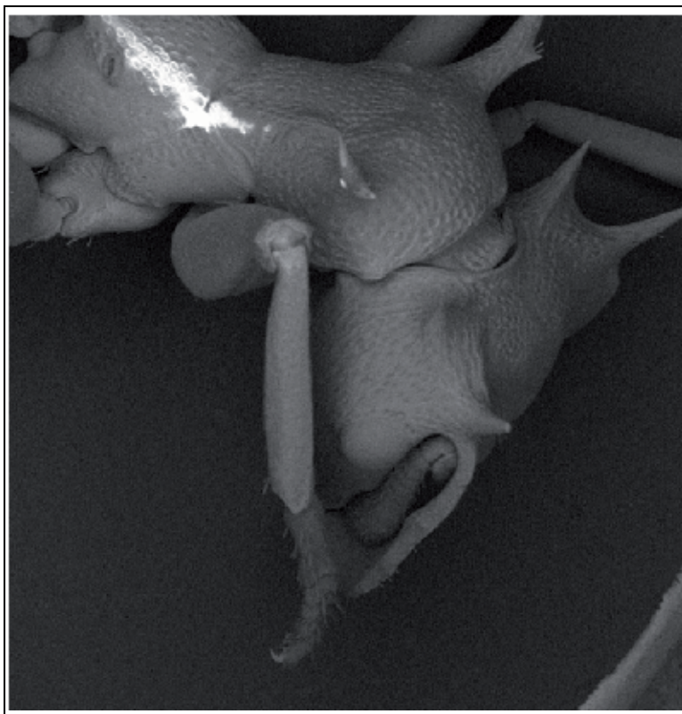
Fig. 2. SEM image of a biological sample(cephalotes) using quad backscattered detector. The sample was not sputter coated resulting in excessive charging(white area) on the sample.
