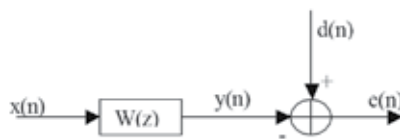
Fig. 10. block schematic of a linear discrete-time filter W(z) for estimating a desired signal d(n) based on an excitation x(n) where d(n) and x(n) are random processes.
