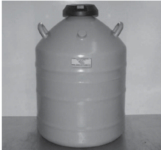
Fig. 4. Liquid nitrogen Dewar vessel, used for freezing and storing cryopreserved oocytes. Courtesy of Reproductive Medicine Associates of New York, LLP.
