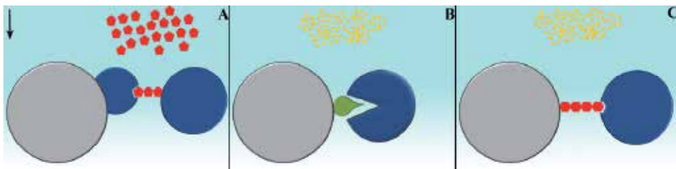
Fig. 2. Illustration of the affinity chromatography methodologies. The target molecules are bound to their ligands immobilized on a solid phase matrix. (A) Lectin affinity chromatography, (B) Protease inhibitor affinity chromatography and (C) Glycosaminoglycan affinity chromatography. Proteins = blue circle; carbohydrates = red pentagon and hexagon; protease inhibitors = green drop-like form; ions = yellow circles; and solid phase matrix beads = gray circle.
