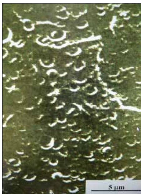
Fig. 3. Surface of COC-blend with designed pores with diameters ranging from 0.6 to 1.5 \mu\text{m}
