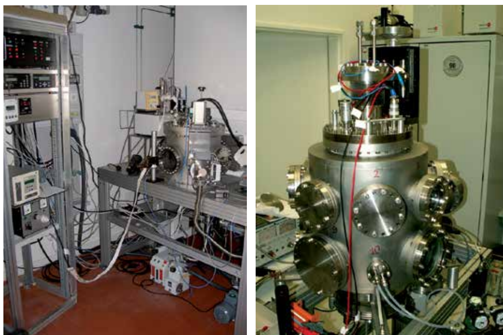
Fig. 1. Laboratory-size low-temperature plasma reactors for argon / ethylenediamine plasma (left) and pulsed magnetron sputtering (right)
