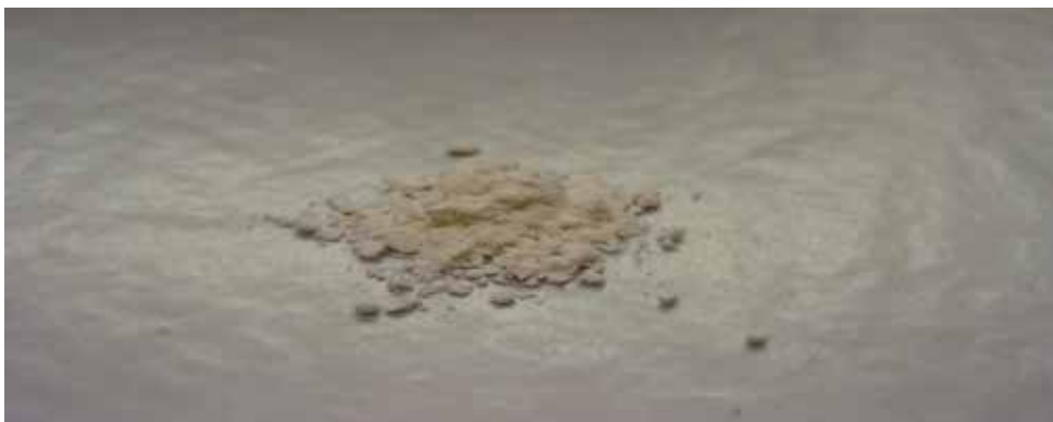
Fig. 9. Particulate SIS. Individual particles in this preparation are no greater than 150 \mu\text{m} in diameter.
