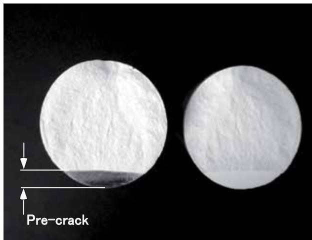
Fig. 5. Photograph of the fracture surface in a HA/Ti specimen after 3point bending test. Note that the crack propagated into HA.
