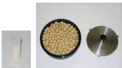
Photo 6. The sample presentation methods for an NIRFlex N-500. (a test tube for a powder, and a dish and a lid for plural seeds)
