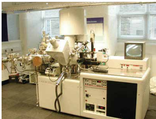
Fig. 9. Kratos Axis Ultra XPS instrument ( http://xps.web.its.man.ac.uk )
