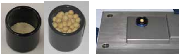
Photo 4. The sample presentation methods for an FT-NIR spectrometry MPA (powder, plural seeds, and a single seed)
