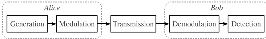
Fig. 5. Diagram of the optical part of a QKD system, where Alice and Bob denote the sender and the receiver, respectively.
