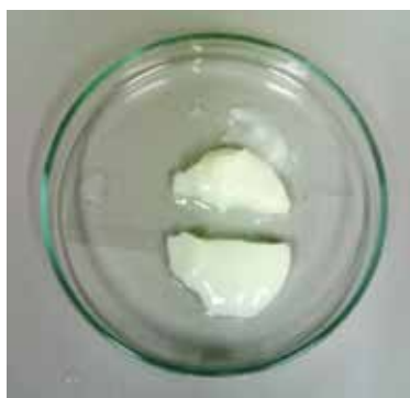
Fig. 3. As-synthesized wet slurry nanoparticles before freeze-drying.
