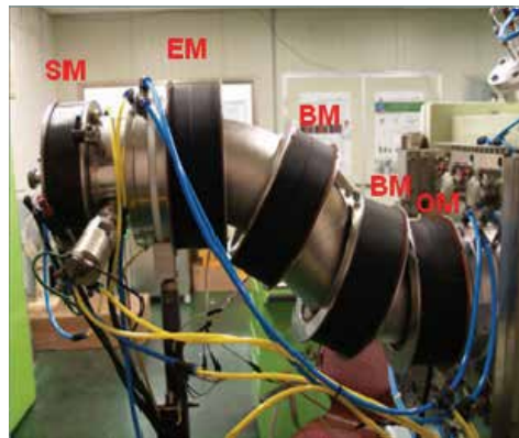
Fig. 3. S-shape filtered vacuum arc system.
