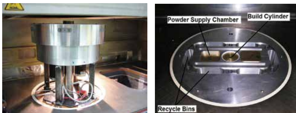
Fig. 20. Modification of Sinterstation ® 2000 system: miniature sintering platform before installation (left) and after installation (right).
