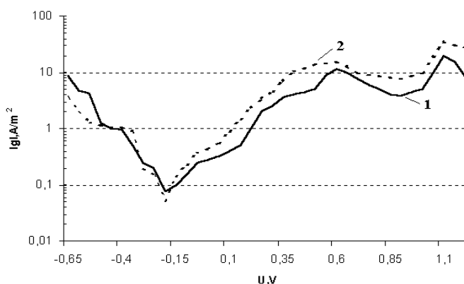
Fig. 22. Polarization curves of oxynitride (1) and nitride (2) coatings on the titanium surface in 80% aqueous solution of sulphuric acid.
