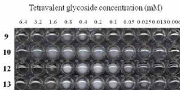
Fig. 6. Photographs of precipitate formed by addition of tetravalent glycosides to WGA-PBS solution.
