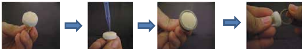
Fig. 4. Procedure step sequence of powdered jack bean immobilization.
