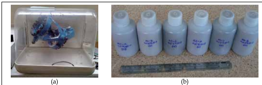
Fig. 5. (a) Turbula mixer used to mix the powders. (b) Powder mixtures.
