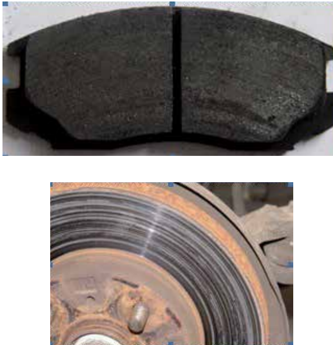
Fig. 16. Post on-road performance test photograph on brake pad and brake disc
