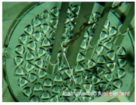
Fig. 19. Core upper view with the instrumented fuel element (Zacarias Mesquita and Cesar Rezende, 2010)
