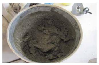
Fig. 2. Fresh state of lightweight mortar prepared with expanded vermiculite aggregate.
