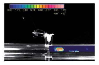
Fig. 6. The visualization data of PIV measurement of 0.050sec after ignition (L/D=18.3 and flame rate=200 f/s,  $\theta$  =30 deg )
