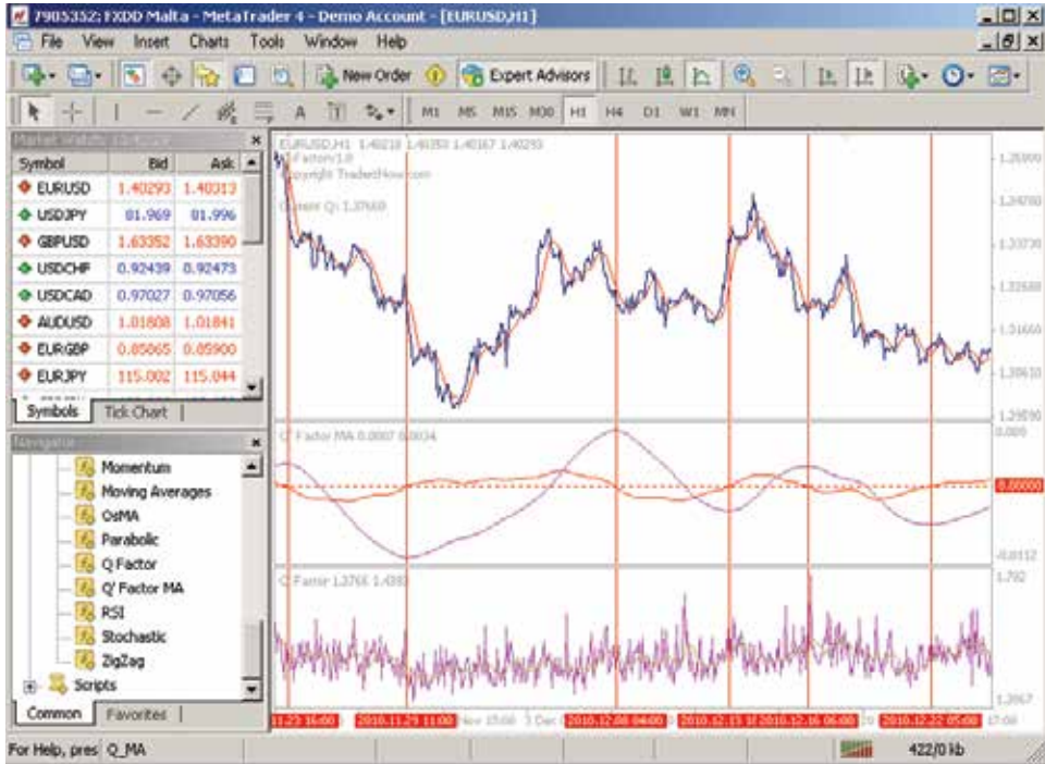
Fig. 4. MetaTrader 4 GUI for new indicators. Top window: Euro-USD exchange rate signal for 1 hour sampled data (blue) and averaged data (red); Centre window: first (red) and second (cyan) gradients of the moving average for (N, M, K, T) = (512, 10, 100, 0) . Bottom window: q_j (cyan) and moving average of q_j (Green).
