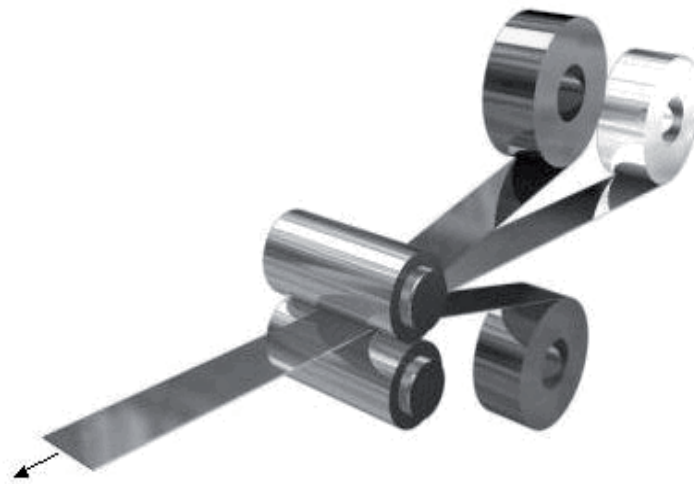
Fig. 24. Principle of roll cladding of a three layer metal composite.
