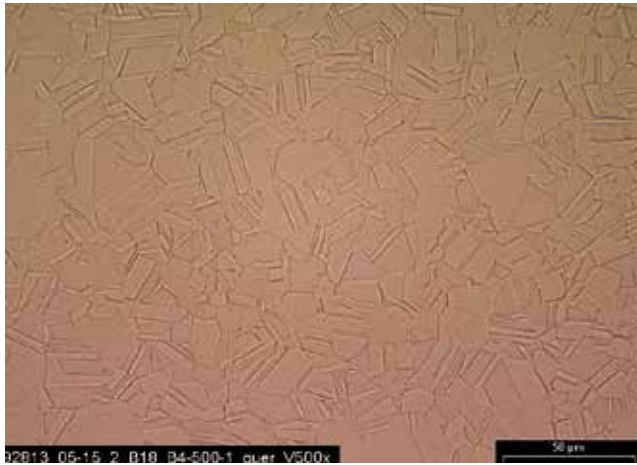
Fig. 13. Microstructure of conventionally processed CuSn8 with 2-4 twins per grain.
