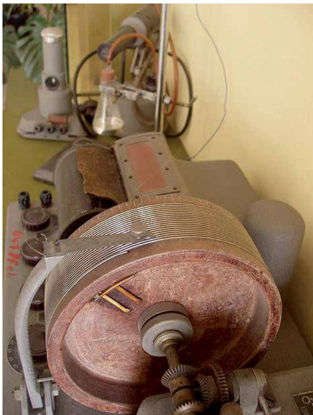
Fig. 4. Heyrovsky's polarography instrument
