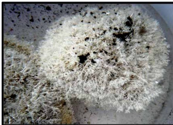
Fig. 14. Another silver dendritic growth with needle-like formation. The black spots on top were holes left by the bubbles ejection.
