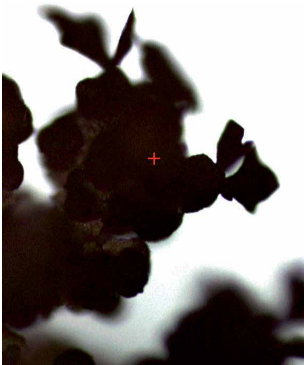
Fig. 10. Image from a lead deposition in an edge of a manganese plate with a semi-dendritic column constituted by grain nucleations and leaves-like forms on top.
