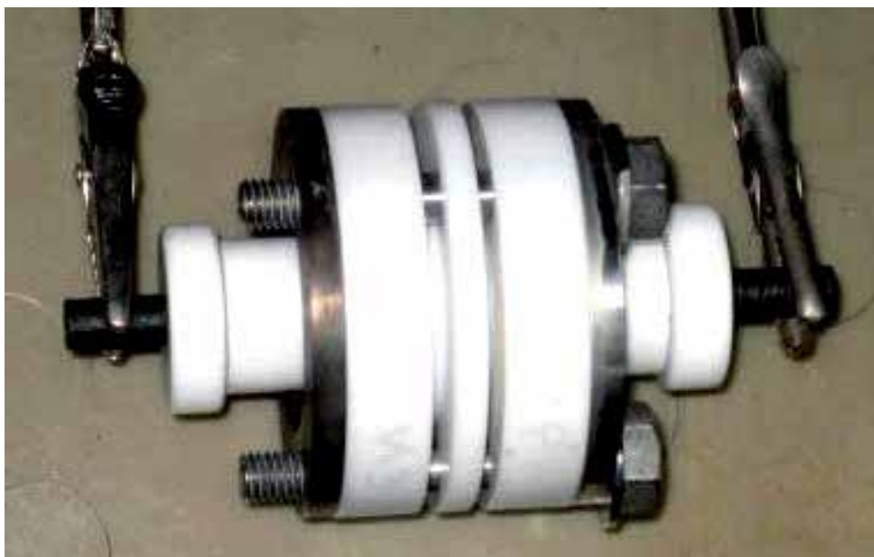
Fig. 2.b Photograph of the electrochemical cell
