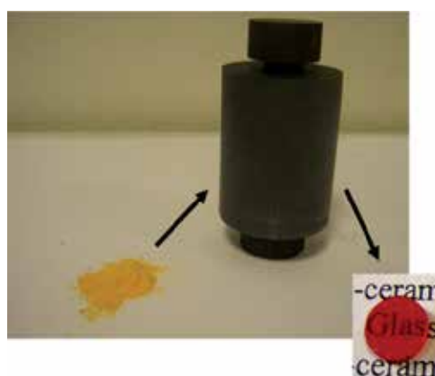
Fig. 10. Photograph of the processed glass sample for the composition 62.5\text{GeS}_2\text{-}12.5\text{Sb}_2\text{S}_3\text{-}25\text{CsCl} .
