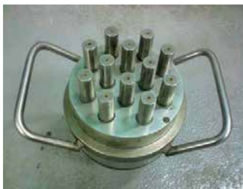
(b) Step 2: To set up the pestle into the mold into the mold
