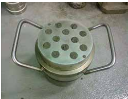
(a) Step 1: To fill the mixed cement-based composite into the mold
