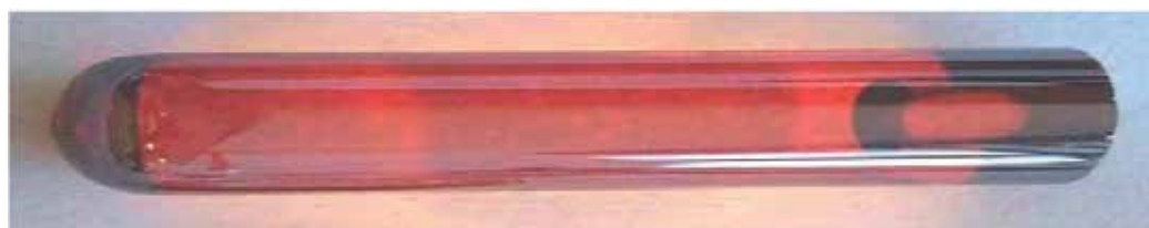
Fig. 2. Example of glass rod of the \text{GeS}_2\text{-Sb}_2\text{S}_3\text{-CsCl} composition.
