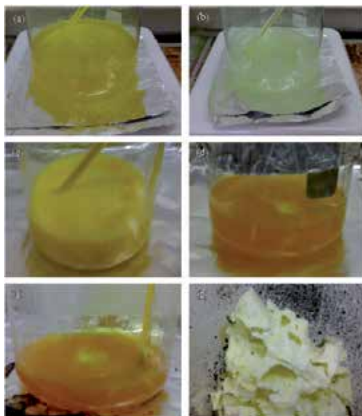
Fig. 1. Evolution of (a) Bi-Ti precursor (b) Pr precursor (c) Bi-Ti precursor stirred at 40°C for 2 hour (d) Bi-Ti precursor heated at 90°C (e) viscous gel and (f) as-combusted powder.
