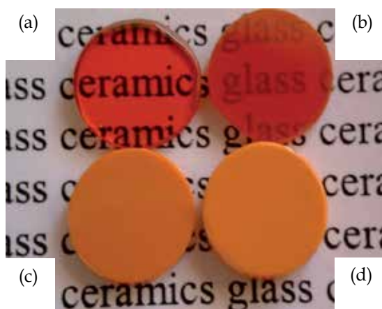
Fig. 5. Glass composition 62.5\text{GeS}_2\text{-}12.5\text{Sb}_2\text{S}_3\text{-}25\text{CsCl} heated at 290^\circ\text{C} for different crystallization times (a) No thermal treatment (b) 7h (c) 73h and (d) 144h.
