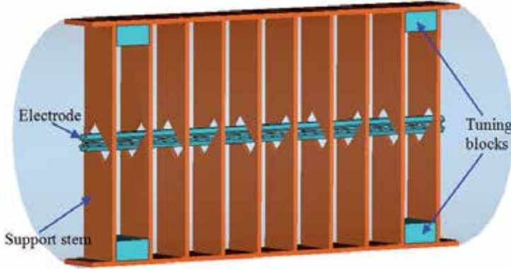
Fig. 4. MWS simulation model of the ladder IH-RFQ.
