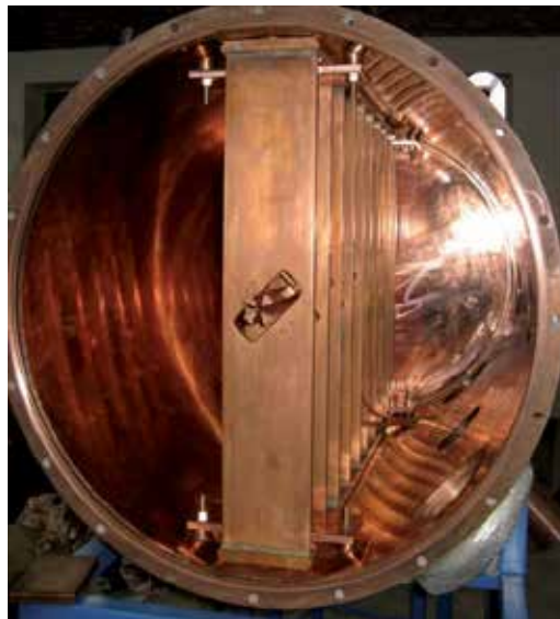
Fig. 10. The constructed ladder IH-RFQ cavity.
