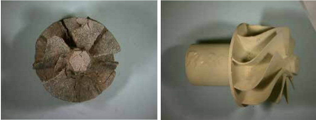
Fig. 23. Turbocharger rotor manufactured from a \gamma -TiAl-alloy after oxidation for 1000 h at 1050°C in air. Left image: Untreated rotor. Right image: Fluorine-treated rotor.
