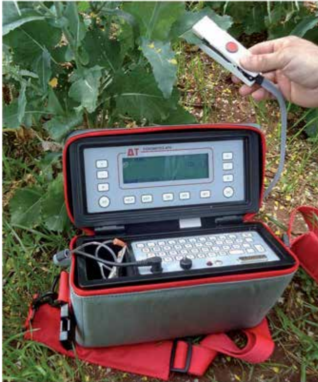
Fig. 9. Stomatal conductance determination using a porometer. Photo: Ana Cláudia Pedersen.
