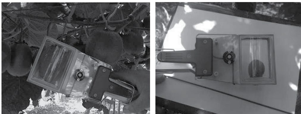
Photo 1. Measurement of fruit transpiration in attached kiwifruit (left) and detached apricot (right) using a portable gas-exchange equipment (ADC-LCA4, ADC BioScientific Ltd, Hoddesdon, England).
