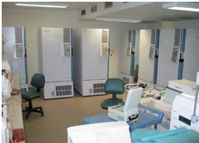
Fig. 3. Mechanical freezers for deep freezing ( -65^{\circ}\text{C} - -80^{\circ}\text{C} )
