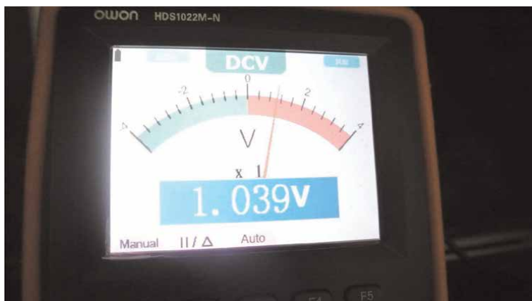
Figure 5. Depending on the geometry of the melanin-based battery, we obtain direct current values such as the one shown in the photograph.
