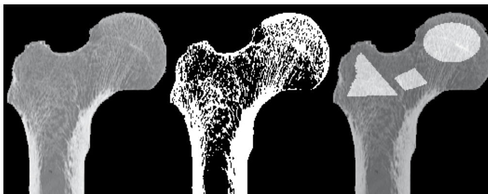
Fig. 1. Left: HRCT image of a human femur specimen with BMD = 0.69 \text{ g/cm}^2 and FL = 3912 \text{ N} (left). Middle: Binarized dataset according to the procedure explained in section 2.5. Right: Visualization of the fitted VOIs: head (ellipsoid), neck (cylinder), and trochanter (irregular) in the original CT data.
