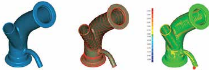
Fig. 9. Results of the tubing example tested using Geomagic , (a) polygon mesh (589,693 triangles), (b) NURB model (1,107 patches), and (c) deviation analysis
