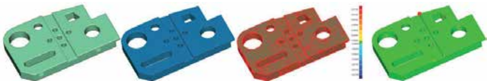
Fig. 8. Results of the block example tested using Geomagic , (a) point cloud model (634,957 points), (b) polygon mesh (1,271,924 triangles), (c) NURB surface model, and (d) deviation analysis
