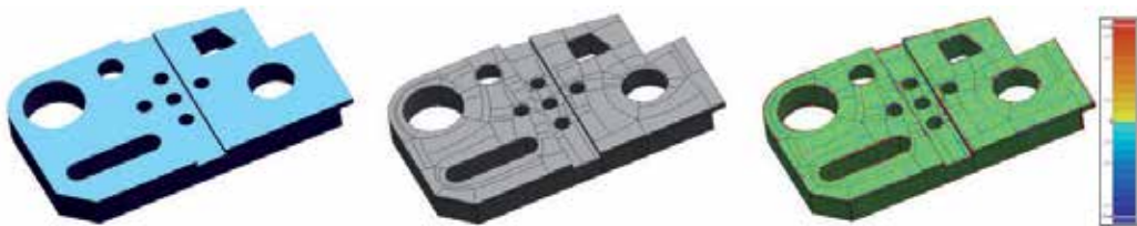
Fig. 12. Results of the block example tested using Rapidform , (a) polygon mesh (1,062,236 triangles), (b) NURB surface model (273 patches), and (c) deviation analysis
