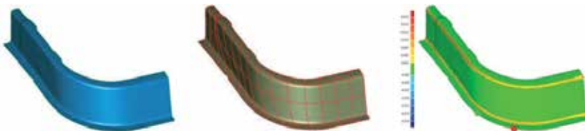
Fig. 10. Results of the sheet metal example tested using Geomagic , (a) polygon mesh (126,492 triangles), (b) NURB model (91 patches), and (c) deviation analysis
