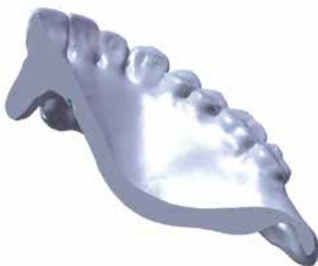
Fig. 12. The third analysis model: the fault is considered near the bottom of the denture
