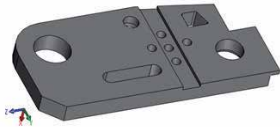
Fig. 22. Block exported from Rapidform to SolidWorks , (a) solid model exported to SolidWorks , and (b) design change made in SolidWorks
